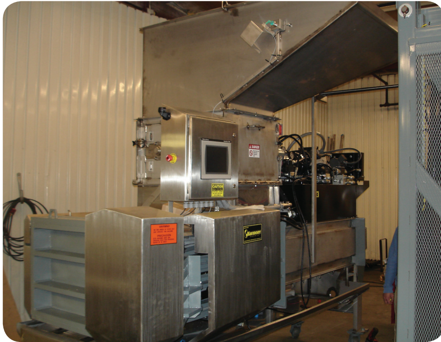
An Allen-Bradley PanelView Plus Compact HMI provides onsite access to machine information.
